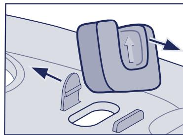
**Remove** filter light from underside of lid before **washing**. Push tab away and lift to **remove** light. **Replace** before using.
